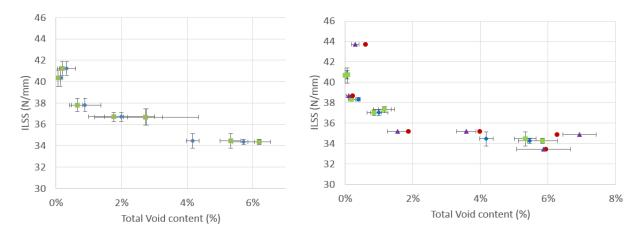
Figure 2: Local measured void content vs. ILSS, averaged across rows (left) and further split into columns (right).
