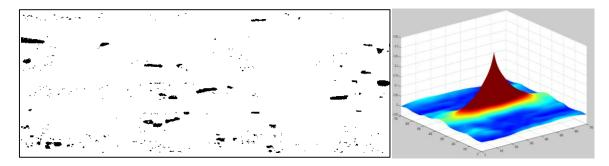
Figure 1: Thresholded micrograph of voids (left), 2-point correlation showing density and directionality of void clusters.
